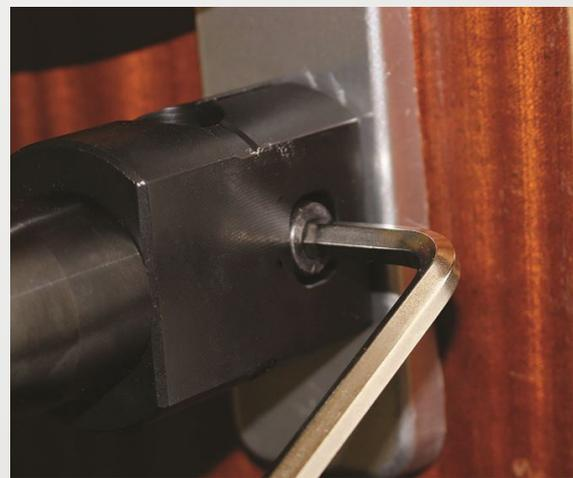
Adjustable clamp to perfectly fit the Souber Snapper onto the cylinder.
