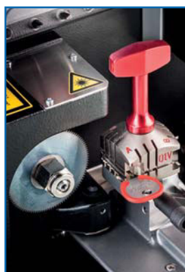
Flat and cruciform key cutting station
